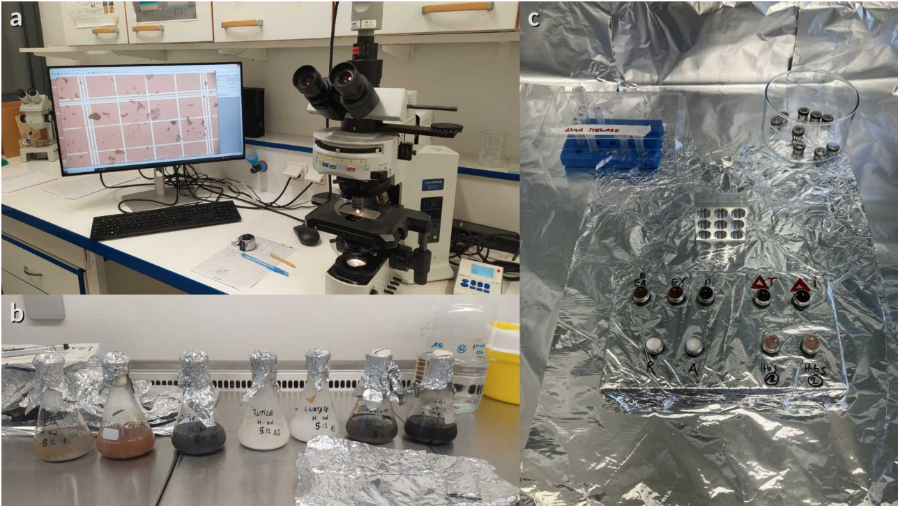
152 153 Figure 1. Laboratory encounters. a) Counting Metallosphaera sedula cells under a microscope. b) 154 Cultivation of Metallosphaera sedula on mineral materials (from left to right: ESA01-E, JEZ-1, pyrite, rutile, 155 anatase, titanium dioxide, and ilmenite). c) Transferred cell-mineral material into metal exposure wells.
